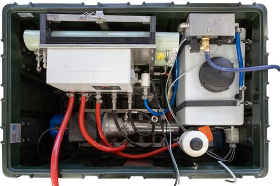
The bespoke design can deliver 450 litres/hour of clean drinking water from a fresh water source and 200 litres/hour from a saline water source.
